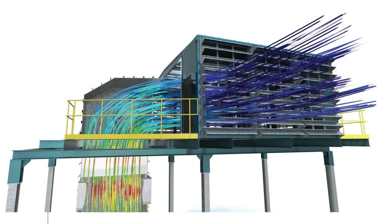
By adding SOLIDWORKS Simulation analysis and SOLIDWORKS Flow Simulation fluid flow analysis software to its SOLIDWORKS Premium design solution, Optar has reduced the time and costs of design simulation and validation, while improving the performance of its air intake filter housing designs, running studies like the fluid flow analysis shown here.
